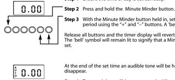
**Step 3** With the Minute Minder button held in, set the required Minute Minder period using the "+" and "-" buttons. A 'bell' symbol will light up.
